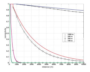
Figure 1: Multihop connectivity in a traffic stream with density=58 veh/km and market penetration rate=10%
