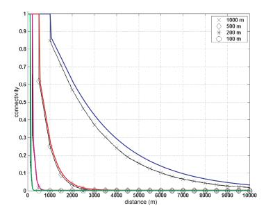
Figure 2: Multihop connectivity in a traffic stream with density=19 veh/km and market penetration rate=10%
